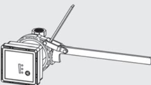
Tighten the union nut with 30 Nm torque.
