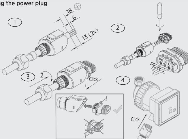
Connect the power cable to the pump as shown. **Caution: Line voltage!** Observe the required protective measures, national body regulations and local provisions at all times. The cable cross-section may no smaller than  $0.75 \text{ mm}^2$ . Use ferrules if using fine-wire cables.
