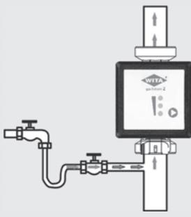
The system must be thoroughly flushed before the pump is started up to prevent contaminants or foreign bodies from remaining in the system.
